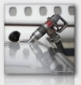
In three separate and distinct instances at locations in the United States, including Nebraska and Florida, over the past three years, DEF has been mistaken for fuel system icing inhibitors (FSII), a clear liquid that is added to aircraft jet fuel.
